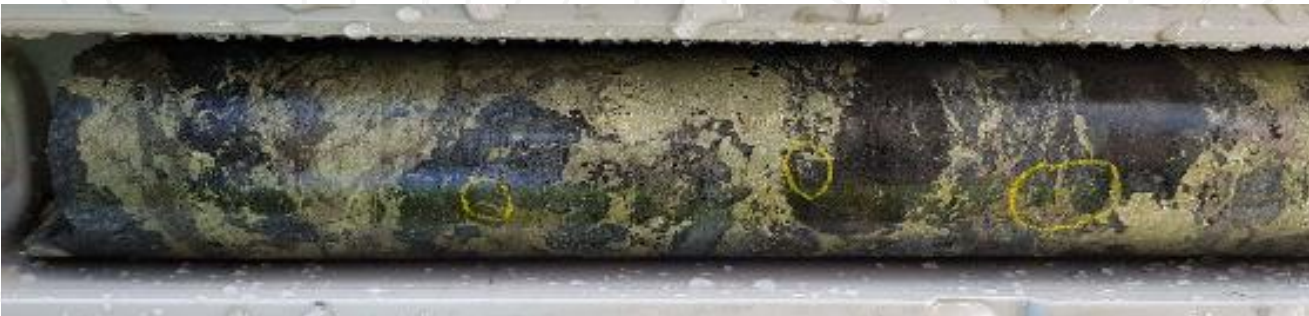
Kanmantoo style Fe-Au-Cu-Bi mineralisation in SLDD001 at 344m
