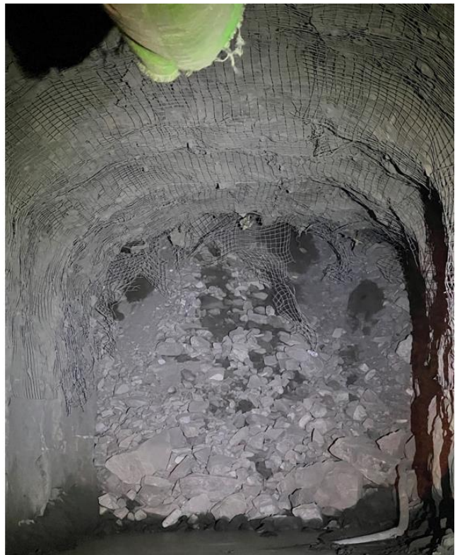
Figure 1 Drawpoint of the first stope (LHS), and close-up showing excellent fragmentation (RHS)
