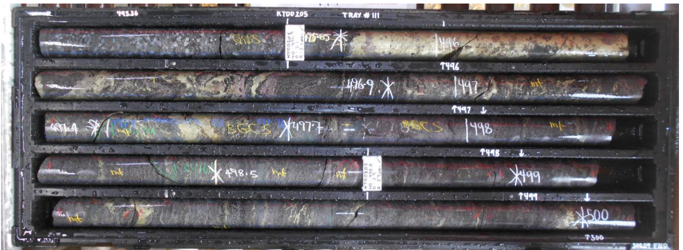
Figure 3 Cu-Au mineralisation in KTDD205 in Kavanagh from 495.36m to 500.09m
