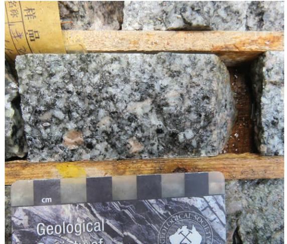
5(d) Medium- to coarse-grained granodiorite observed in the Tongchang pit. (Photo 418099)
