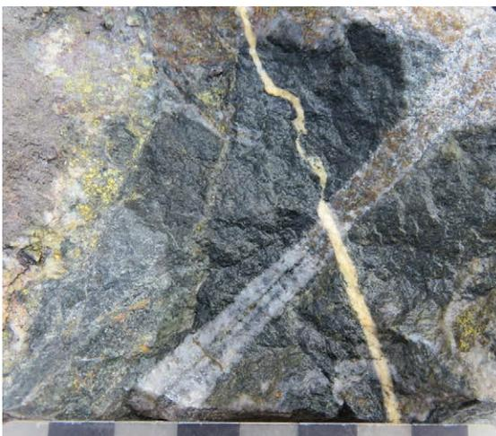
5(e) Dark mafic micro-enclaves with possible basaltic composition cut by quartz–pyrite–molybdenite vein and a late stage calcite vein observed in the Tongchang pit. (Photo 418100)
