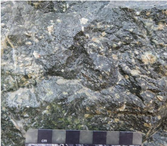
5(c) Sericite-altered porphyritic granodiorite observed in the Tongchang pit. (Photo 418098)
