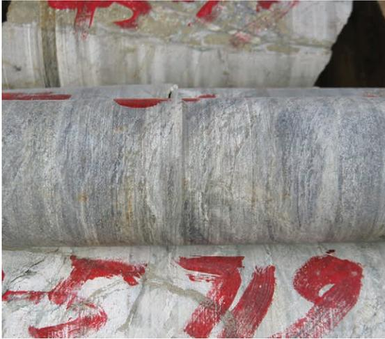
5(a) Example of sheared metasedimentary unit of the Zhangcunyan Group in drill core distal to the Dexing porphyry system. (Photo 418096)
