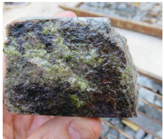
5(f) Intense epidote–quartz alteration and chalcopyrite within the granodiorite from drill core. (Photo 4181001)
