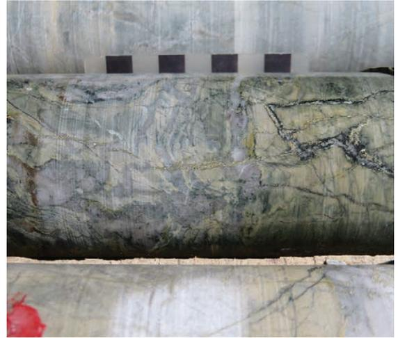
5(b) Intensely fractured metasedimentary rock with pyrite-rich veinlets. (Photo 418097)
